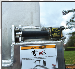
E-Z latch with oval-shaped stop/turn/tail light
